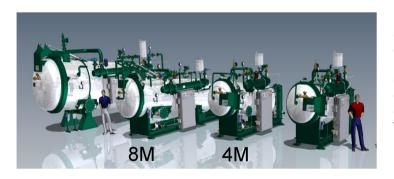
Every RIDA system comes with a performance guarantee that it can achieve a microbial inactivation of STAATT¹ Level IV, which translates to a reduction of bacterial spores by at least a factor of 1,000,000:1, commonly referred to as  $6\log_{10}$  or  $10^6^2$ . This level is considered "sterilization." Some competing units which are rated for STAATT Level III achieve a reduction factor of 10,000:1, which is considered only "inactivation."
